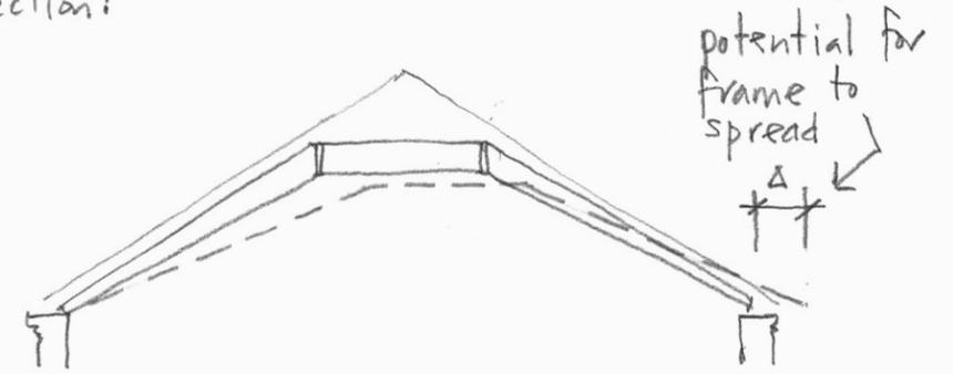
structure designed to work as beam but roof geometry means that 'spread' will occur under loading... this could be eliminated by providing cable ties... or allowing movement to happen.
