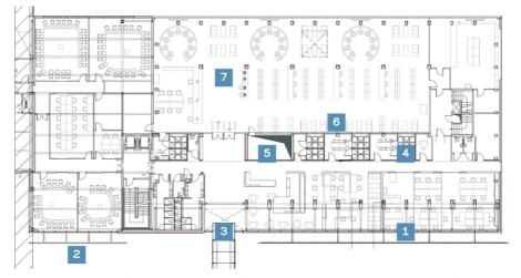
1 Mesh cladding system 2 Projection screen 3 Entrance 4 Ventilation chimneys and lightwells 5 Ventilation chimney/service riser 6 Circulation wall running length of building 7 LRC area
