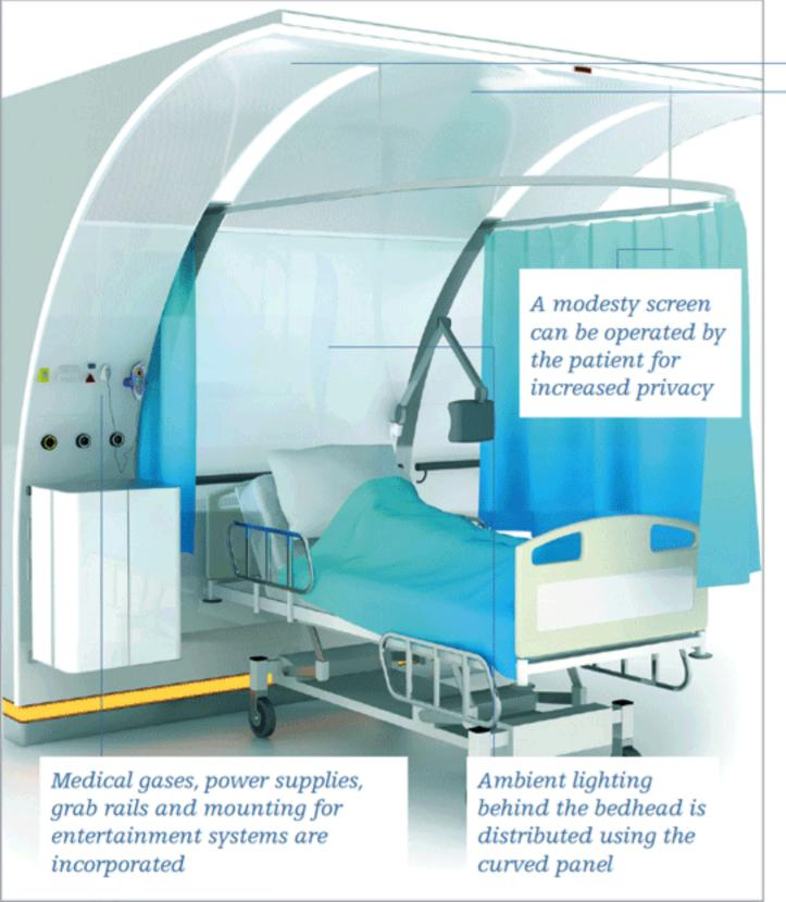
Curved perforated metal bedhead and ceiling canopy redirects sound down to the bed reducing the volume of conversation between a patient and clinician by up to 20dB Low level LED lighting gives patients enough light to safely navigate around the ward at night when general lighting levels are reduced
