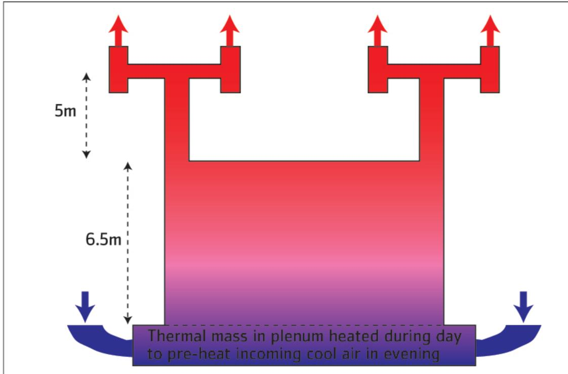
Concept - displacement ventilation when warmer inside figure 1. Design of natural ventilation system at the Contact Studio
