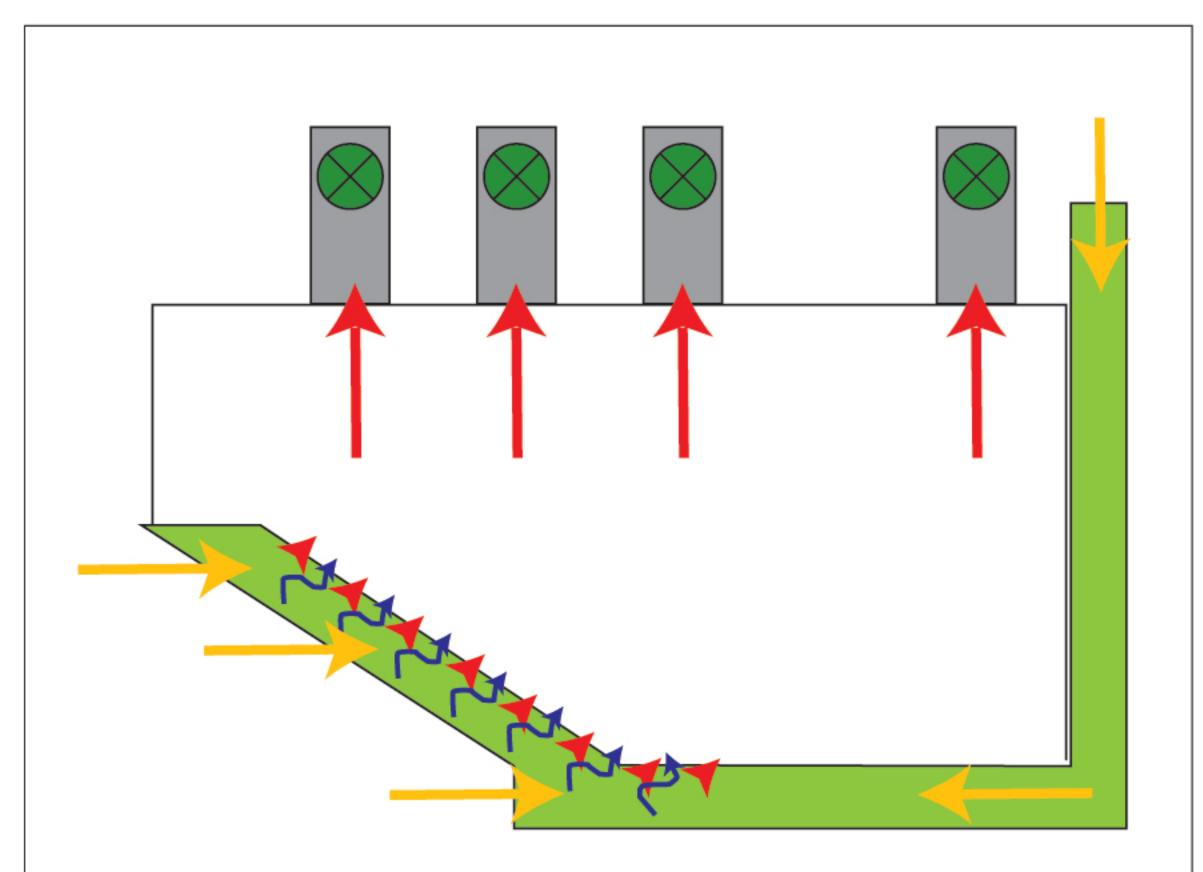
figure 3. Schematic of the proposed up-flow displacement ventilation design for the Garrick Theatre at Lichfield. This section illustrates four of the eight outflow stacks which were designed on the roof of the theatre. It also illustrates the inflow through the thermally massive plenum and through a down-draught stack
