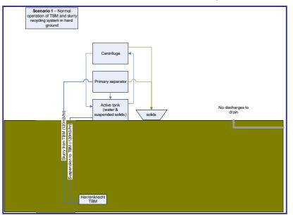
allows a fully closed system that does not generate any effluent for disposal (see diagram Scenario 1).
