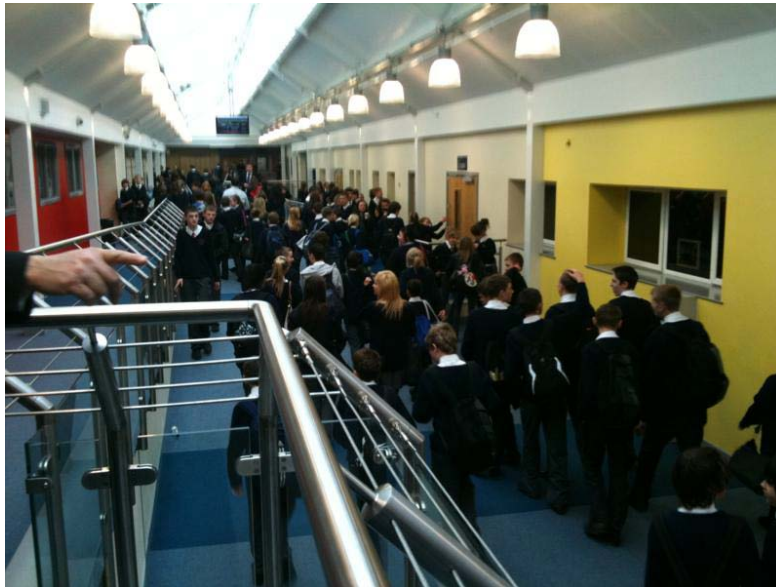
Fig 17: At Temple Moor High School, roofing over the space between existing blocks to create a top-lit walkway allowed students to move between lessons without jostling, listening to music instead of a school bell.
